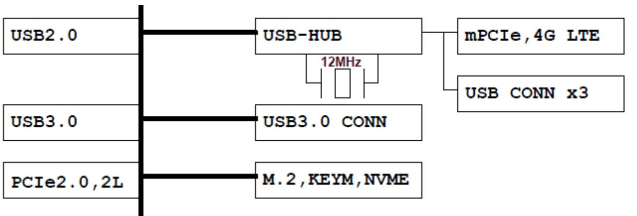
mPCIe slot is usb-only with SIM connector (bottom of board). PCIe is mapped to m.2 key-m slot for nvme SSD
